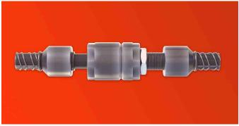
This particular coupler may be connected to the rebar by conventional means or by friction welding as detailed earlier. The adjustable coupler is typically used for connection of precast elements where each part of the coupler may be cast in-situ in each precast element. Connection in this way allows for the adjustment on site of the eventual connection ensuring tight tolerances are met.
