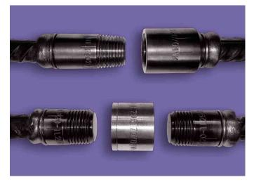
After cutting square, the ends of the bar may be enlarged, or "upset", by cold forging, such that the core diameter of the bar is increased to a predetermined diameter. A parallel thread is then either cut or rolled onto the enlarged end. Using this technique, the effective diameter of the threaded bar is equal to the bar diameter thereby creating the conditions to promote failures within the bar and not the coupled joint. The coupler is usually assembled using a torque wrench.
