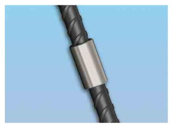
After cutting square, the ends of the bar may be enlarged, or "upset", by cold forging, such that the core diameter of the bar is increased to a predetermined diameter. A parallel thread is then either cut or rolled onto the enlarged end. Using this technique, the effective diameter of the threaded bar is equal to the bar diameter thereby creating the conditions to promote failures within the bar and not the coupled joint. The coupler is usually assembled using a torque wrench.
