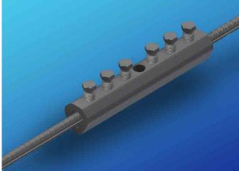
Each end of the bar is inserted into opposite ends of a steel sleeve which is then bolted in a prescribed manner to ensure controlled penetration into the bar surfaces. The couplers are installed with a pneumatic or electric power tool. The bolt heads will shear off when proper installation tightness has been reached.
